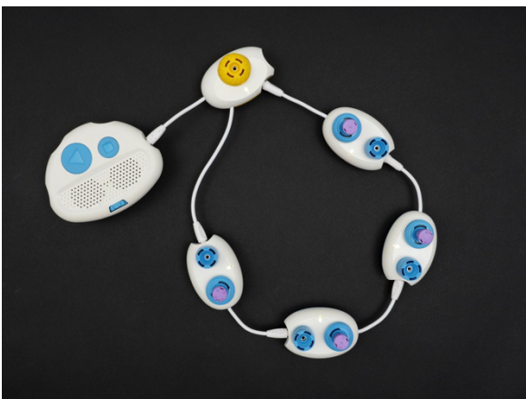
[Figure Caption:] The photo on the left displays a Code Jumper program containing four Play pods, one Loop pod, and four Constant plugs. One Constant plug is connected to each Play pod's Sound dial. The Loop pod is connected by its shorter wire directly to the Hub at Port 1. The Play pods are connected, one after the
